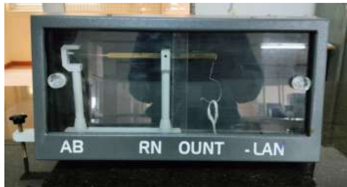
PLATE 3: BEESLEY BALANCE YARN COUNT TEST
